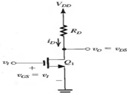
22 If the amplifier is biased to operate with an overdrive voltage  $V_{OV}$  of  $0.5\text{ V}$ , find the incremental gain at the bias point.
