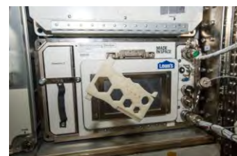
Fig. 2.2.1. 3D printer designed by the company MadeInSpace installed on the ISS (Credit: MadeInSpace)
